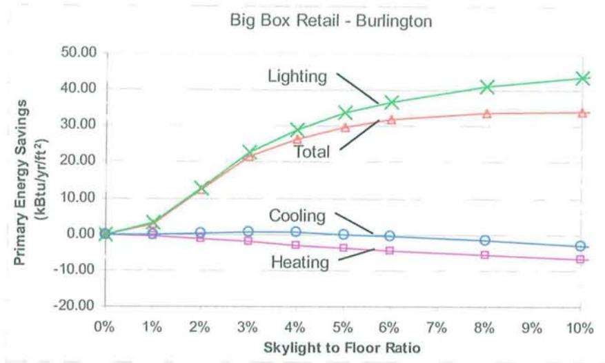
Figure 5-2: Annual Primary Energy Savings by End Use (lighting, cooling, heating) as a Function of SFR, Burlington
