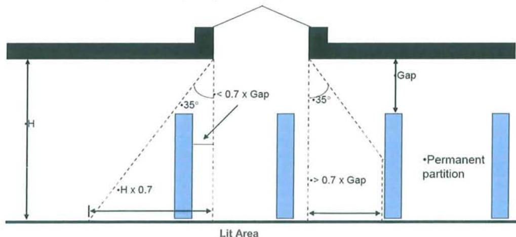
Figure 4-1: Skylight Spacing Criteria (PG&E 2006)
