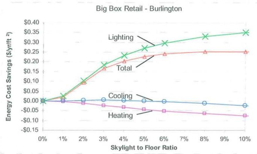
Figure 5-3: Annual Energy Cost Savings by End Use (lighting, cooling, heating) as a Function of SFR, Burlington
