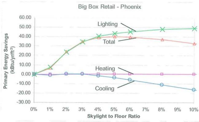
Figure 5-4: Annual Primary Energy Savings by End Use (lighting, cooling, heating) as a Function of SFR, Phoenix
