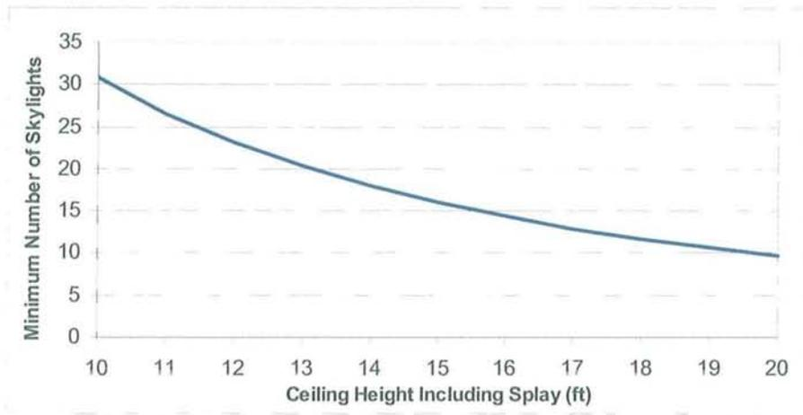
Figure 4-2: Number of Skylights Required for a 10,000 ft<sup>2</sup> Area Versus Ceiling Height
