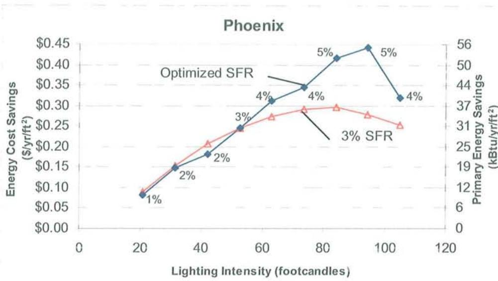
Figure 4-4: Energy Cost Savings as a Function of Required Lighting Intensity / Lighting Power Density, Big Box Retail, Phoenix
