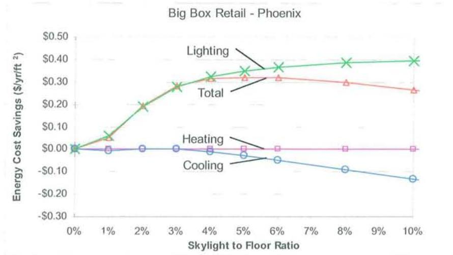
Figure 5-5: Annual Energy Cost Savings by End Use (lighting, cooling, heating) as a Function of SFR, Phoenix
