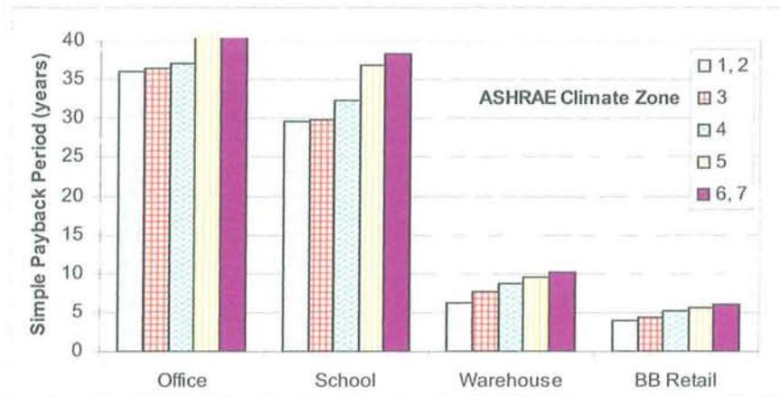
Figure 1-1: Simple Payback Resulting From Energy Savings, by Climate Zone and Building Type
