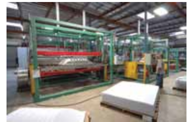
Thermal forming Sunoptics' high-performance prismatics.
